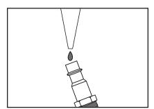
Figure 12. Lubricating nailer via air inlet.
